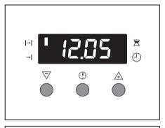
When the time has elapsed, the function indicator flashes, an audible signal sounds for 2 minutes and the oven switches itself off.
